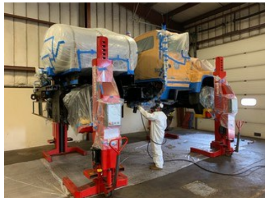
Public Works: DPW worker Kevin Lowery installing the rust-inhibitive paint on a Township's plow/salt brine dispensing truck
